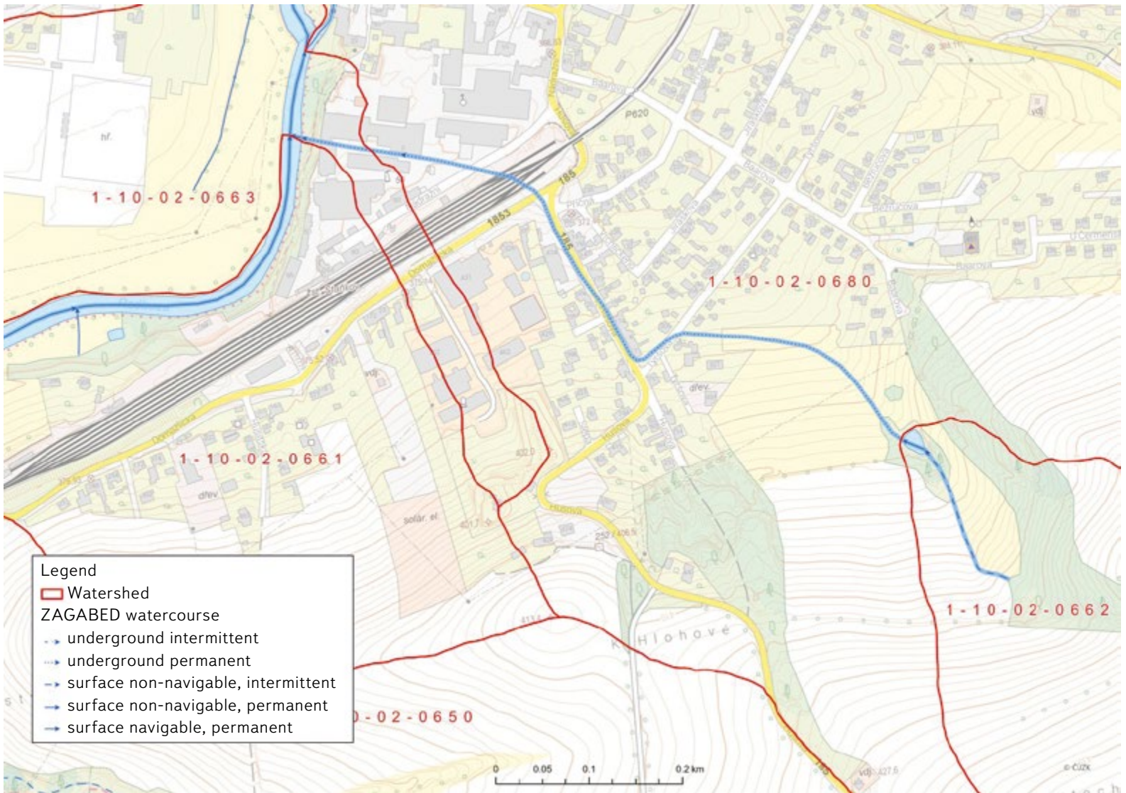
Fig. 1. Example where the drainage divide respected an underground section of a watercourse (dotted blue line)
