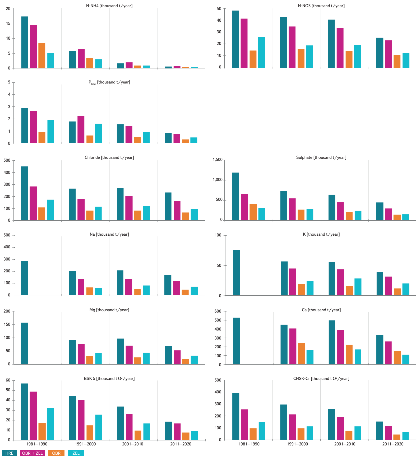
Fig. 2. Ten-years means of transport through monitored profiles in thousand tons per year; second column represents the sum of transport/supply by Elbe and Vltava at the confluence
